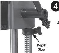
4. Raise the head using the Operating handle to the top of its travel, and hold in place by securing the Depth Stop.
