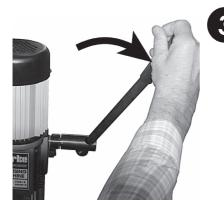
3. The handle is used to raise and lower the head. It may be repositioned for maximum leverage and comfort during operation.
