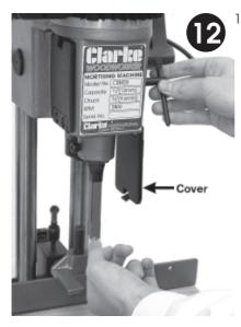
Push the drill bit up through chisel, and into the opened jaws of the chuck as far as it will go, then back off approx. 1/16"(2mm).
