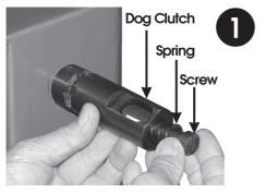
1. Attach the Dog Clutch to the Raise/Lower spindle in the manner shown - thread the spring on to the screw stem then, screw it into the spindle through the hole in the dog clutch and tighten fully.
